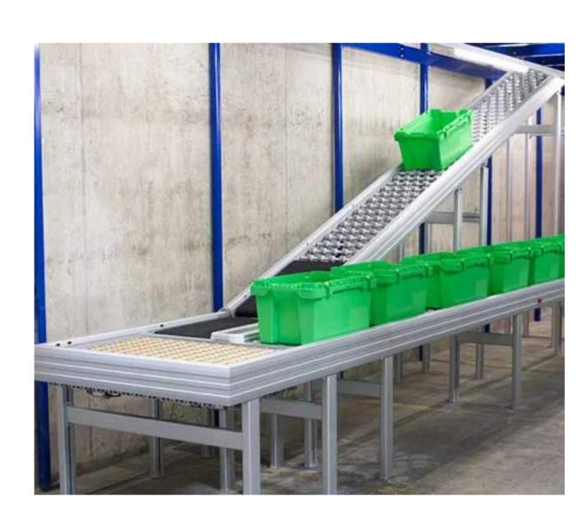
Avancon has effectively shattered this paradigm with the introduction of roller conveyors equipped with softer polyurethane tires (70° shore), mirroring the versatility of belt conveyors on inclines and declines of up to approximately 20°. Not only do these roller conveyors facilitate the seamless transportation of items with flat bases, but they also offer the added benefit of pressure-less accumulation on any incline or decline, further enhancing operational efficiency.
