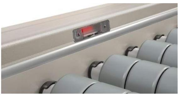
If a zone is occupied, the motor is switched off to save energy; if it's free, the motor is activated, swiftly moving materials to available zones. Thus, the entire system can transport goods quickly, reaching speeds of up to 1.5 m/s while consuming only 40 to 80 W of energy per unit.
