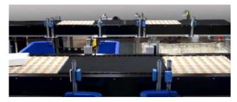
Avancon's OTU stripes are renowned for their ability to facilitate smooth and precise omnidirectional transfers. The OTU's unique design allows parcels to be moved in any direction with minimal friction, ensuring that items of varying shapes and sizes are handled with care and efficiency. This technology is particularly beneficial in high-speed sorting environments where accuracy and speed are essential.
